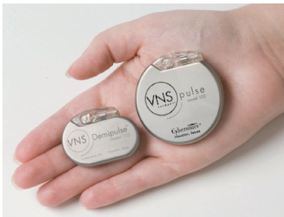
FIGURE 67-2 A model 103 generator (left) next to a model 102 generator (right) demonstrating decreased size.
