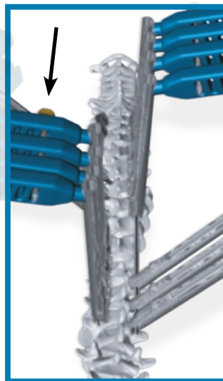
Step 2: Slide linkage rods through handles.
