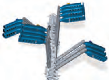
Handle Linkage Rods Are Attached Thru The Handle Of Each Cluster
