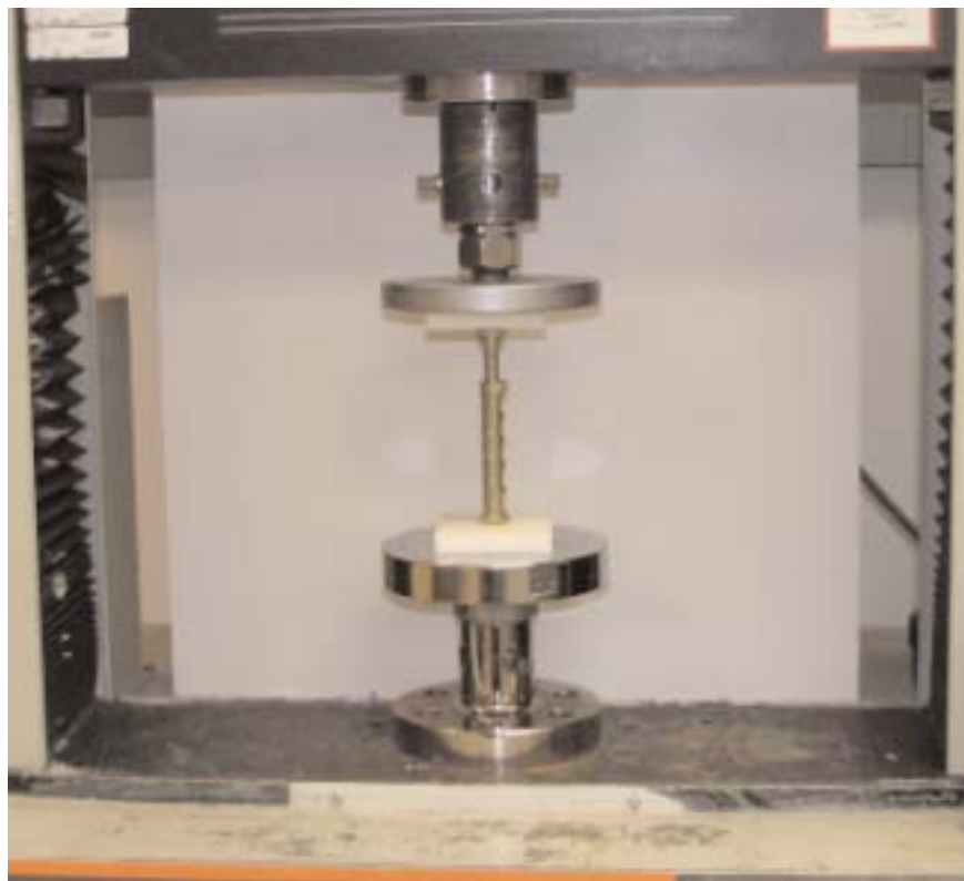
Figure 2. Test setup in Instron 5500R test frame for axial compression of X-MESH.
